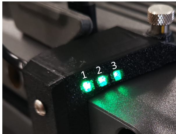
Figure 3.1 – Numbered LEDs on cable
